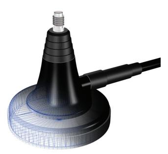
MidiMag has a slim design but is still robust. It has an easy detachable cable with FME connection if you should prefer another cable than the 4.5 m LL58 it comes with. The connection is protected with shrinking tubing.
